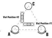
Keep about half the length engaged. When the bubble is centered (**Vial Position #1**), turn the instrument and observe the vial (**Vial Position #2**). Now center the bubble in **Vial Position #2** using only screw  $\mathbf{C}$ . The instrument should now be leveled, but to be certain, double-check. Rotate the instrument  $180^{\circ}$  so the vial is reversed. If the bubble will not center when reversed, follow adjustment procedure outlined under "**Bubble Adjustment**."
